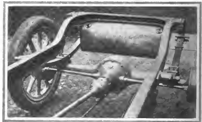
Full floating axle of Newton light car. Note neat brake control
